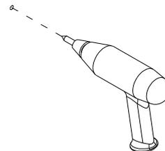
Drill holes at the marks with an electric drill
